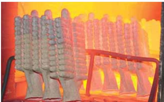
*Ceramic moulds are heated in preparation for casting.*
