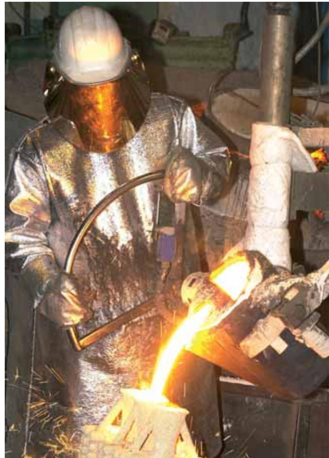
*Molten metal is poured into the mould.*
